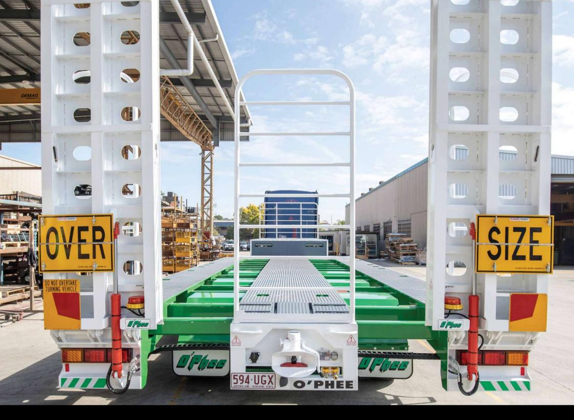
Unique heavy duty 'Widening' frame with ONE-PIECE Gooseneck web.
