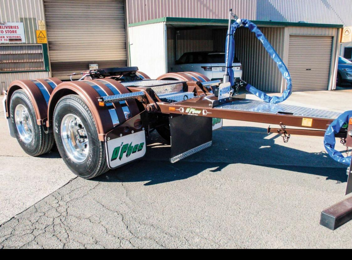
Unique build Triple Rated main Frame-RHS frame strapped side & underside.
